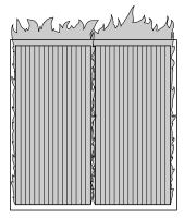
Figure 21 - Incorrect Burner Flame Pattern (Model VN10A Shown)
